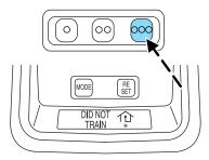
5. Press and hold the just-trained HomeLink® button and observe the HomeLink® house icon on the display. If the indicator light(s) underneath the house icon are constant, programming is complete and your device should activate when the HomeLink® button is pressed and released. **Note:** To program the remaining two HomeLink® buttons, begin with step 2 in the "Programming" section — **do not** repeat step 1.
